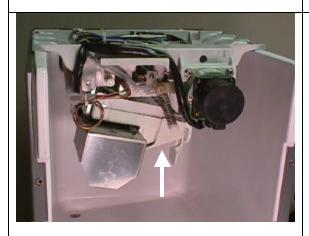
Switching the actuator toggle switch to the left position also reverses the actuator motor. The motor now turns clock wise to raise the water plate upward.
